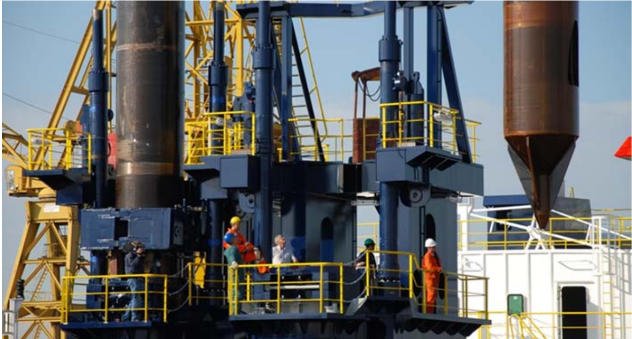
Above seen the installation of the spudcans onboard the newbuilding dredger QUIBIAN I at the IHC-Merwede shipyard in Sliedrecht – Photo : Jan van Heeteren ©
