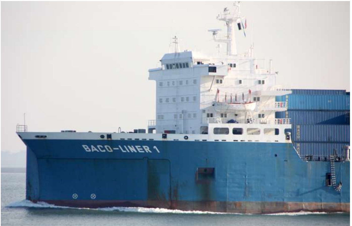
Barge Carrier " BACO-LINER 1 " seen outward bound Westerschelde passing Terneuzen. Delivered in 1979 by Thyssen Nordseewerke GmbH with yardnumber 457. The ship equipped with bowdoors and ramp can carry 501 TEU in cluding 78 ref.containers and 12 lighters/barges. Loa x Lbp x B x D x d: 203,89m x 195,00m x 28,50m x 11,26m x 6,651 - 22.349 GT - 21.801 TDW.
