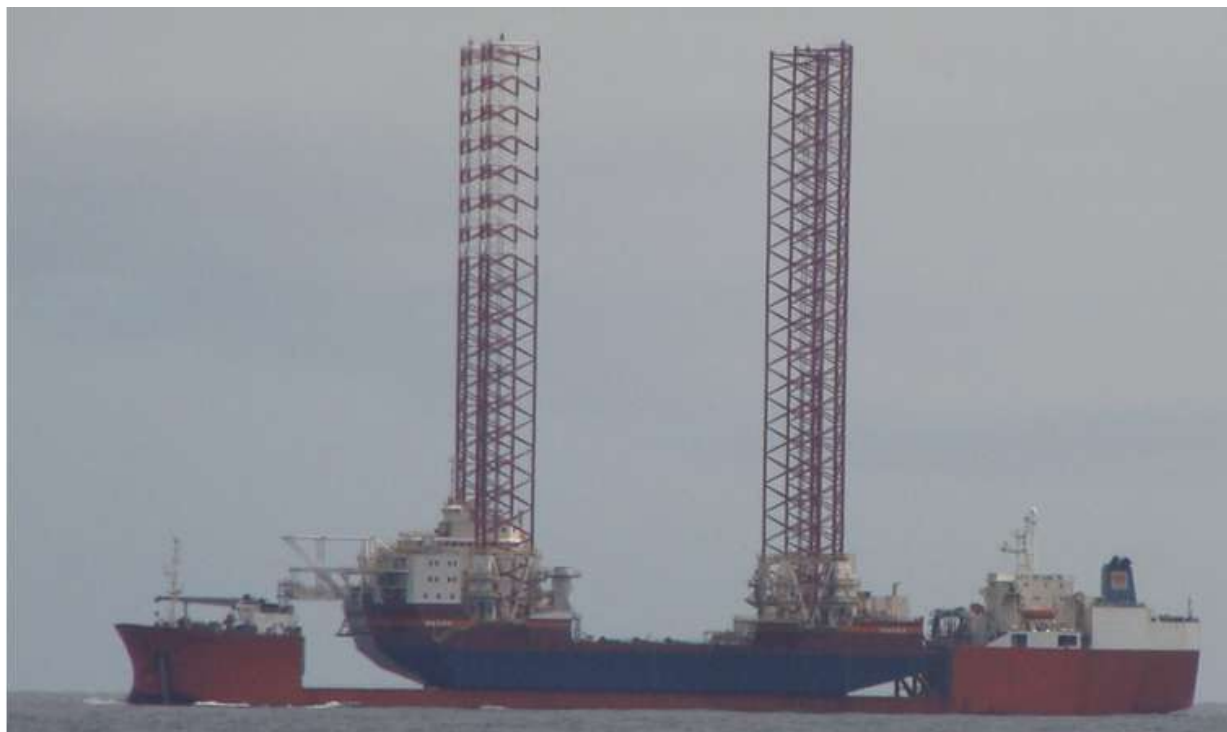
The TREASURE seen near the river Elbe loaded with the jack up platform HAVEN – Photo : Jacob Versteeg ©
