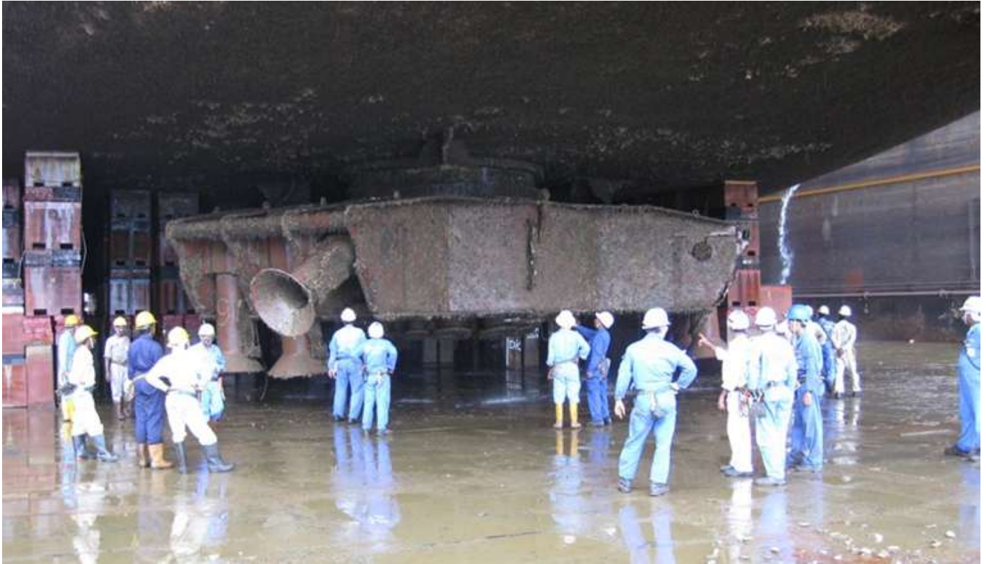
The turntable/turret seen of Bluewater's GLAS DOWR , which entered the drydock at Sembawang Shipyard last week Photo : Bluewater Energy Services BV ©
