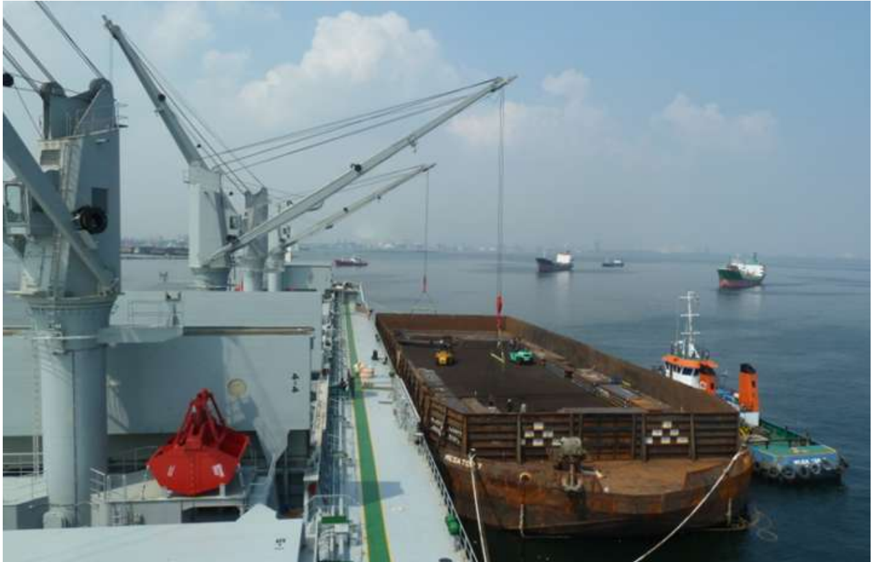
Above seen the discharging operation of a grounded bulker off Tj Priok (Jakarta) several hours before the bulker was successfully refloated and safely anchored by the salvage team - Photo : Piet Sinke (c)
