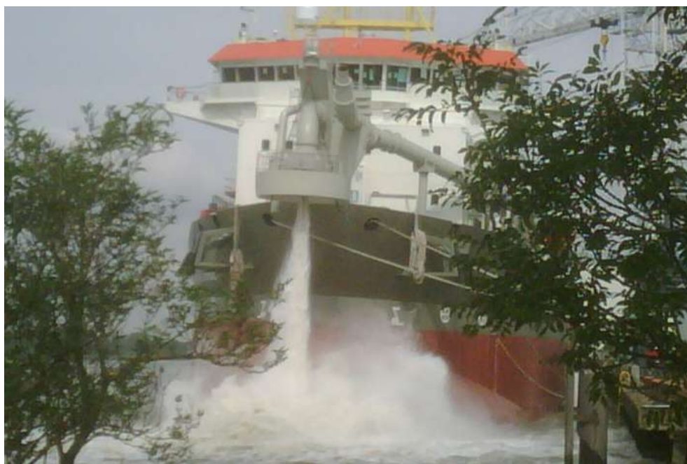
Above seen the new TSHD Willem van Oranje seen during testing of het pump and main engines, the dredger will depart Monday from the builders, IHC-Merwede, for one week yard trials
