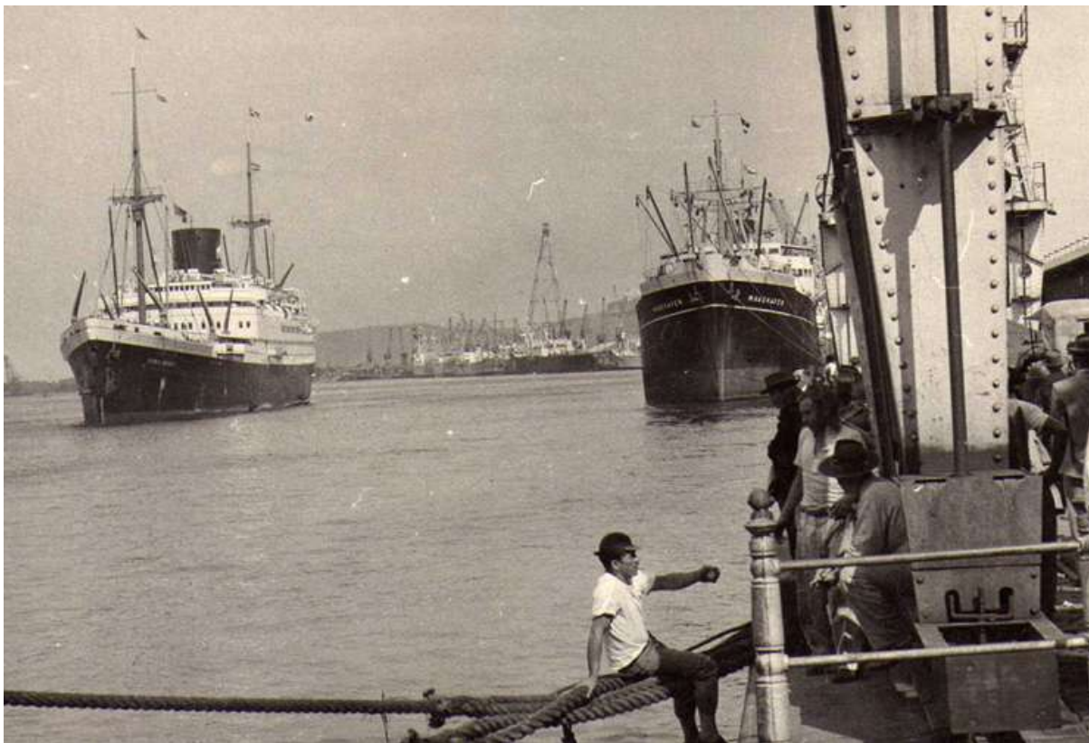
The M/S TEGELBERG seen arriving in Port of Santos-Brazil in 1958 with on the right seen moored alongside the MAASHAVEN , The TEGELBERG was built during 1938. Gross tons: 14.285; length: 559 ft; beam: 72 ft; draft: 30 ft. Speed: 16 kt. Propulsion: Diesel triple screw. Passengers: 131 first class, 84 second, 169 third. - End service: 1968.
