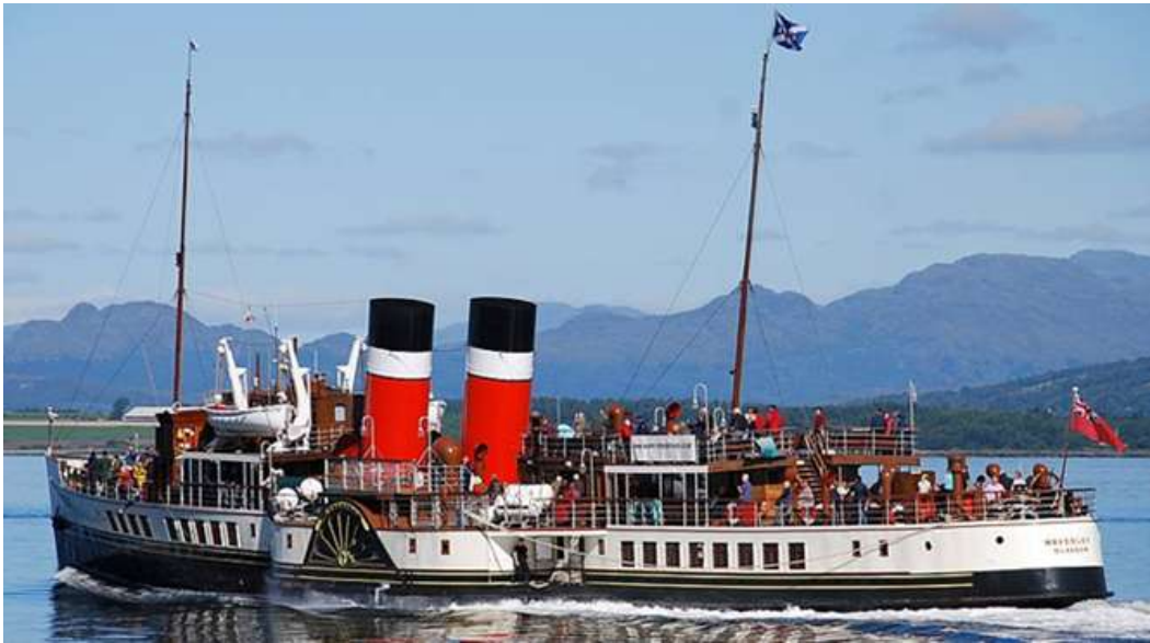
The WAVERLEY is the last Seagoing paddle steamer in the world, seen outbound passed East India Harbour, Greenock. at 11.57 to-day 30/8/2010. She was built by A & J Inglis Ltd, Glasgow in 1947 Yrd No 1331, 693grt. Licensed to carry 950 unberthed passengers. Photo : Iain Forsyth ©
