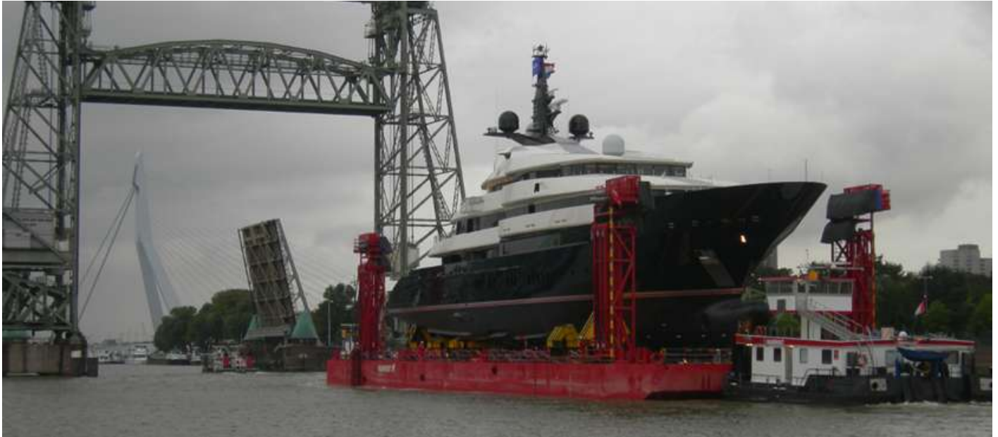
Above seen Mammoet Maritime transport executing the transport of a newbuild yacht (Y 706) from OCEANCO (Alblasserdam) to the Waalhaven for discharging, above is seen the pontoon SCHELDE passing the several bridges in Rotterdam city . Photo : Jos Leentvaar - MAMMOET Maritime B.V. ©
