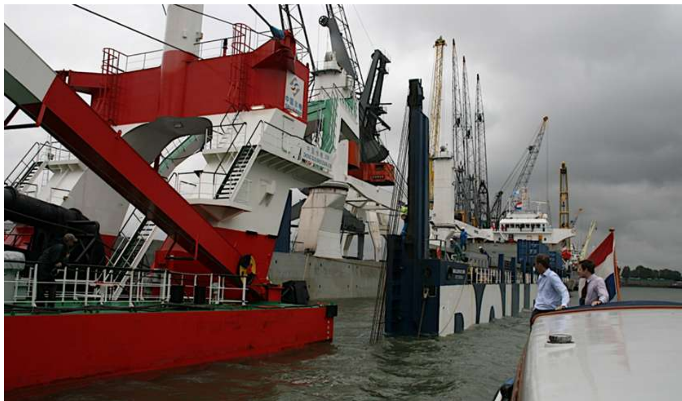
The " Rolldock Sun " executing the float-in operation of the 106 meter long dredger " Zhong Guo Shui Dian J08 " seen from " De Maze ". - Photo : Carlo Jansen (c)
