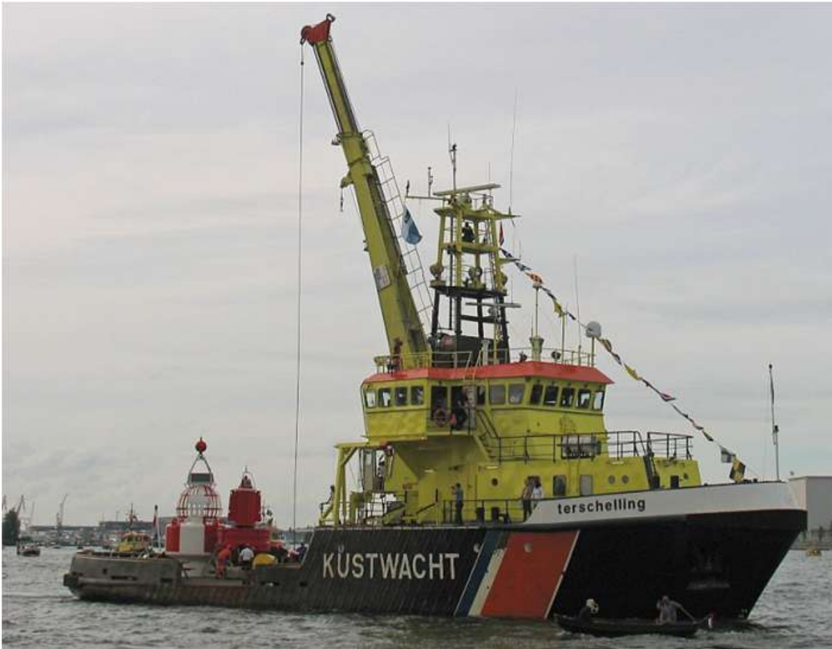
The buoy tender TERSCHELLING seen installing several navigation buoys for the SAIL 2010 event Photo : Willem Kruit (c)
