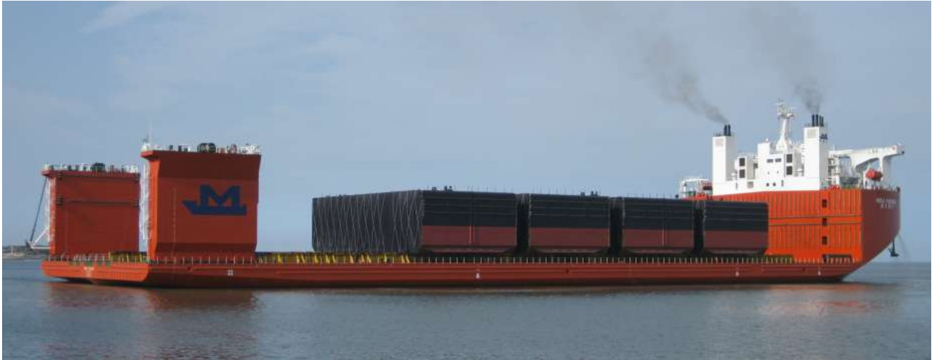
The Semisubmersible heavy cargo carrier " Megapassion " seen departing from Yantai with 4x ~2000mT ring sections for Heerema's H-591 Launchbarge which is currently under construction at DSME in Okpo S.Korea."
