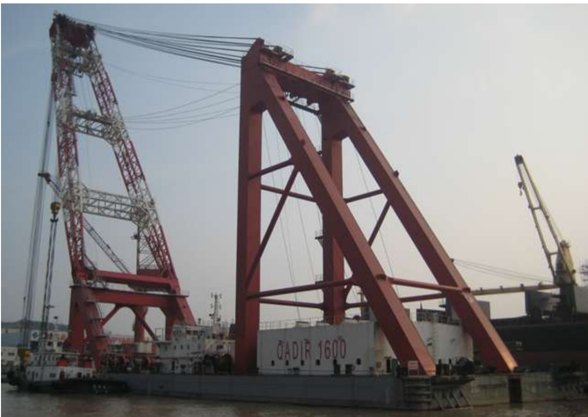
Above seen the 1600 tons shearlegs Zhen Fu 8 , the shearlegs is assisted by the tug Zhen Hua Tuo 11 . Both units are having the ZPMC logo's in the funnel, and installed the last few days several sections in the drydocks in China
