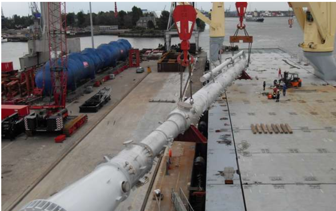
M/V Frauke (SAL) seen loading at Mammoet Terminal Schiedam an 68 mtr Tower being 155 ts with destination Shanghai, China - Photo - B. Stoof COLI Shipping & Transport bv ©
