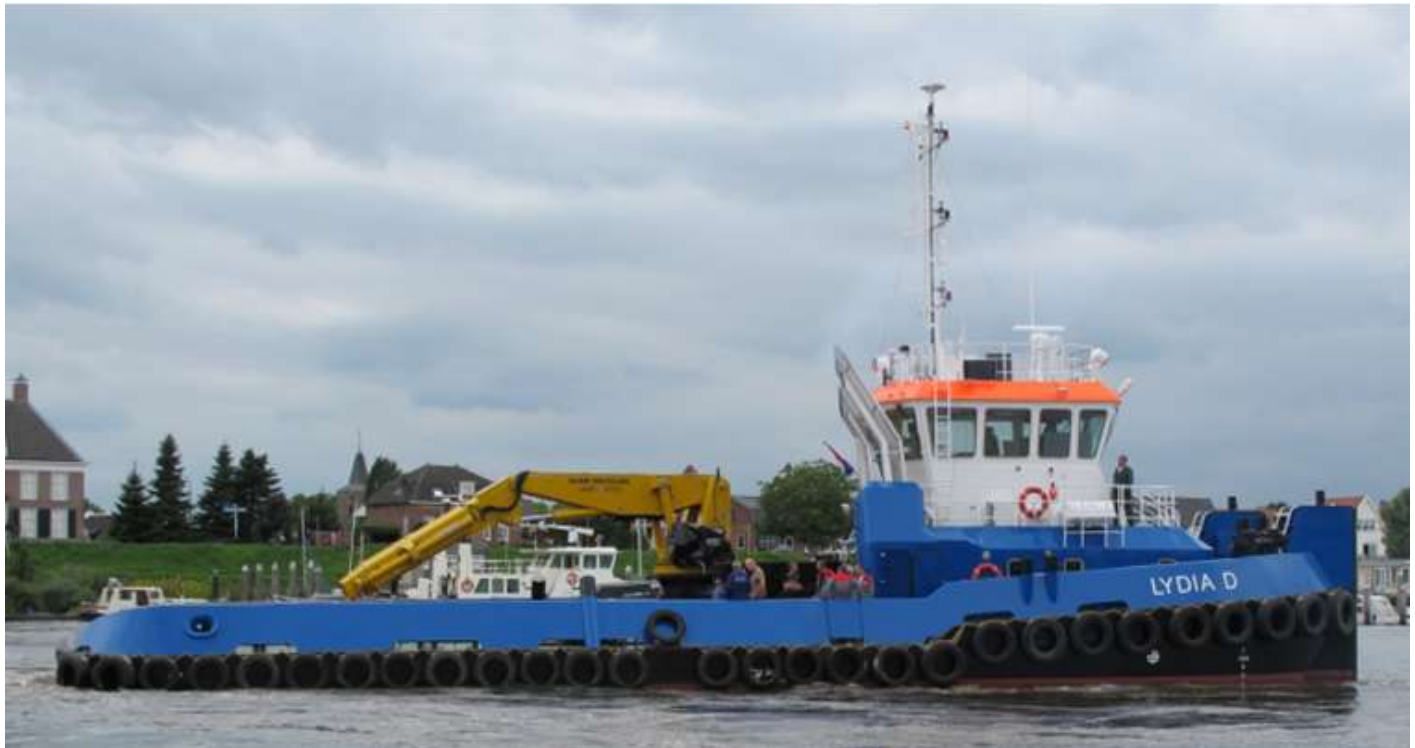
The NEPTUNE SHIPYARD (AALST) built LYDIA D commenced her yard trials, the 31.05 mtr long and 10.00 mtr width workboat is powered by 2 Caterpillar 3512 B HD main engines
