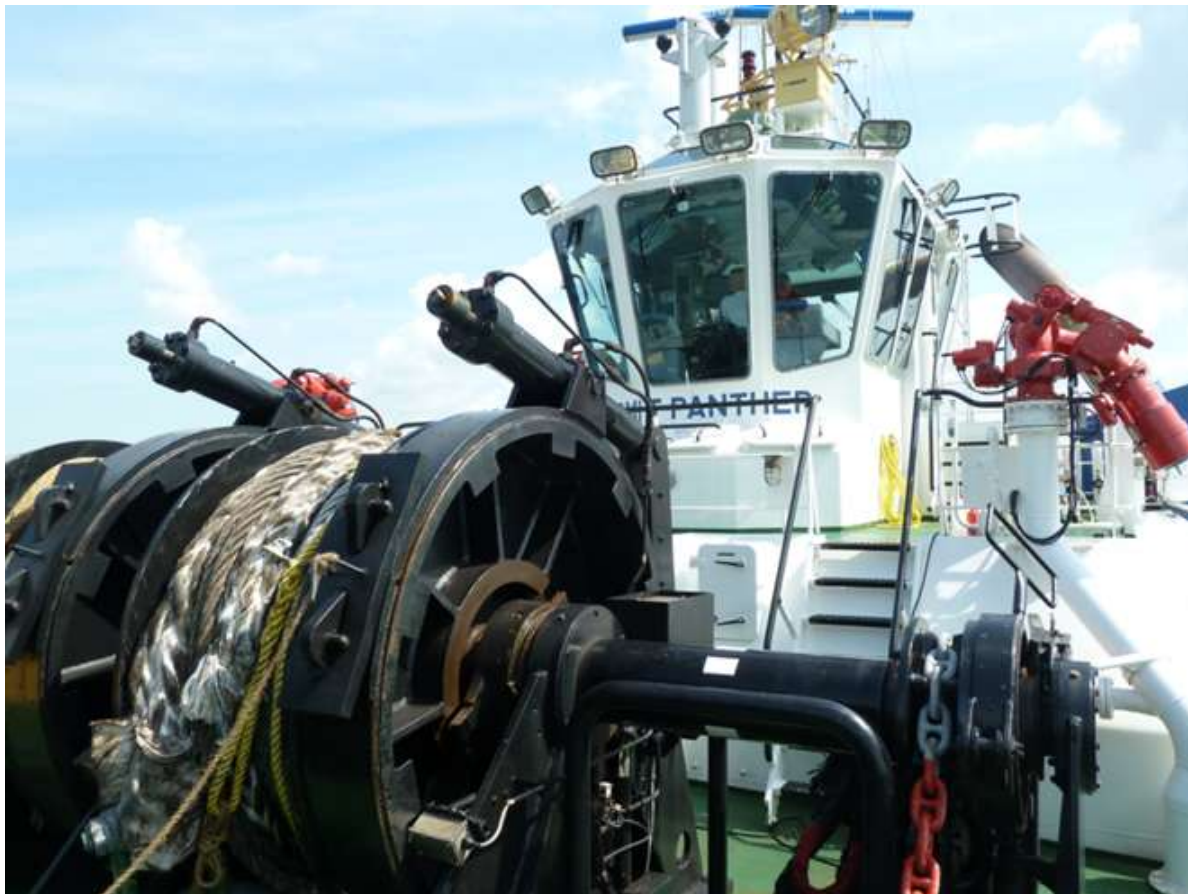
The (bow) towing winch onboard the 95 ton BP SMIT PANTHER which is operating in Rotterdam-Europoort Photo : Piet Sinke (c)
