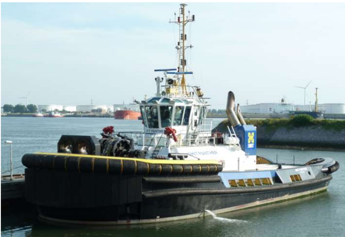
The 95 ton bollard pull tug SMIT PANTHER seen moored in the Scheurhaven Rotterdam - Europoort Photo : Piet Sinke (c)
