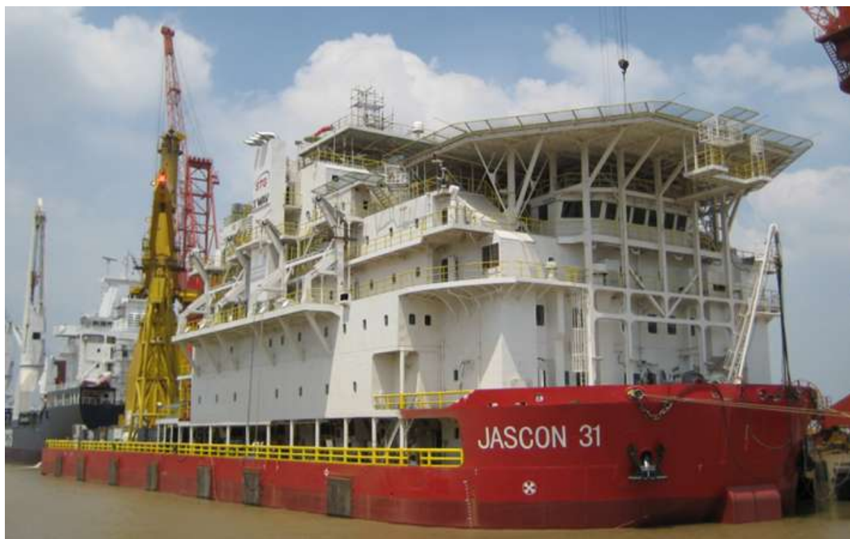
The JASCON 31 seen fitting out at the Juisheng Shipyard (China), installed is an 400T OMC Huisman crane - Photo : Bart Klos (c)
