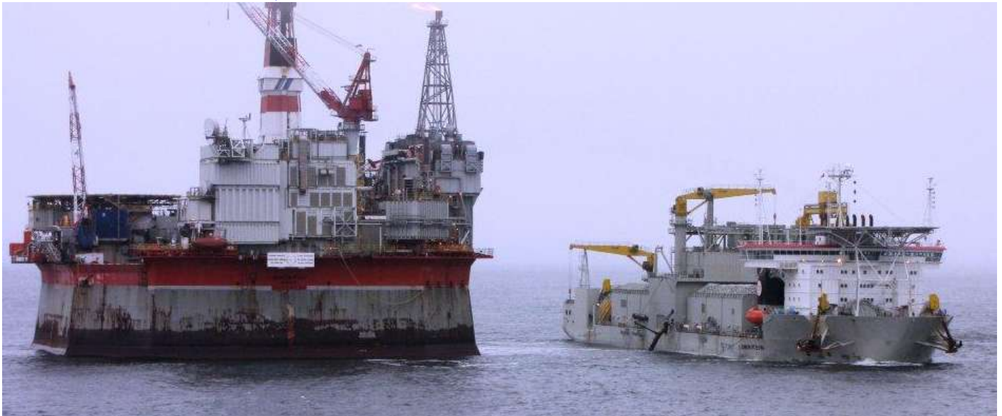
Above and below seen Jan de Nul's SIMON STEVIN operating near the Russian island Sakhalin, the vessel is seen dumping stones / rocks at the foundation of the MOLIPAQ platform and over the pipelines
