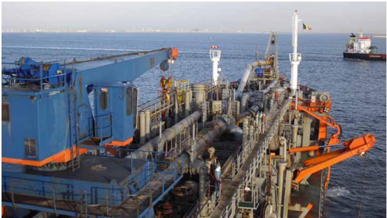
Geopotes 14 seen operating in the Scheldt off Zeebrugge (Belgium) to dredge a trench for the new export cable from the Belwind windfarm - Photo : Capt Theo Haegens – Geopotes 14 ©
