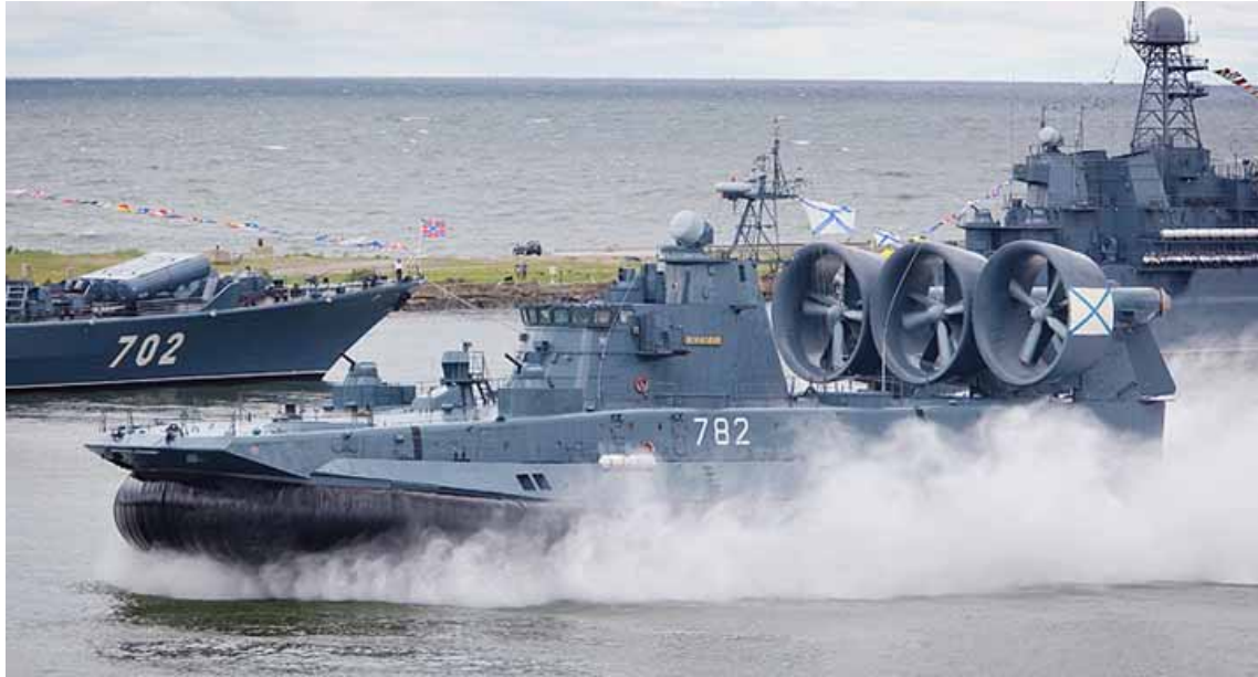
Photo made last weekend in Baltiysk of the 1991 built POMORNIK (ZUBR) class MDK-94 during the Russian navy days 2010, with a 415 tons displacement this air-cushion vehicles are able to achieve a tops speed of 63 knots
