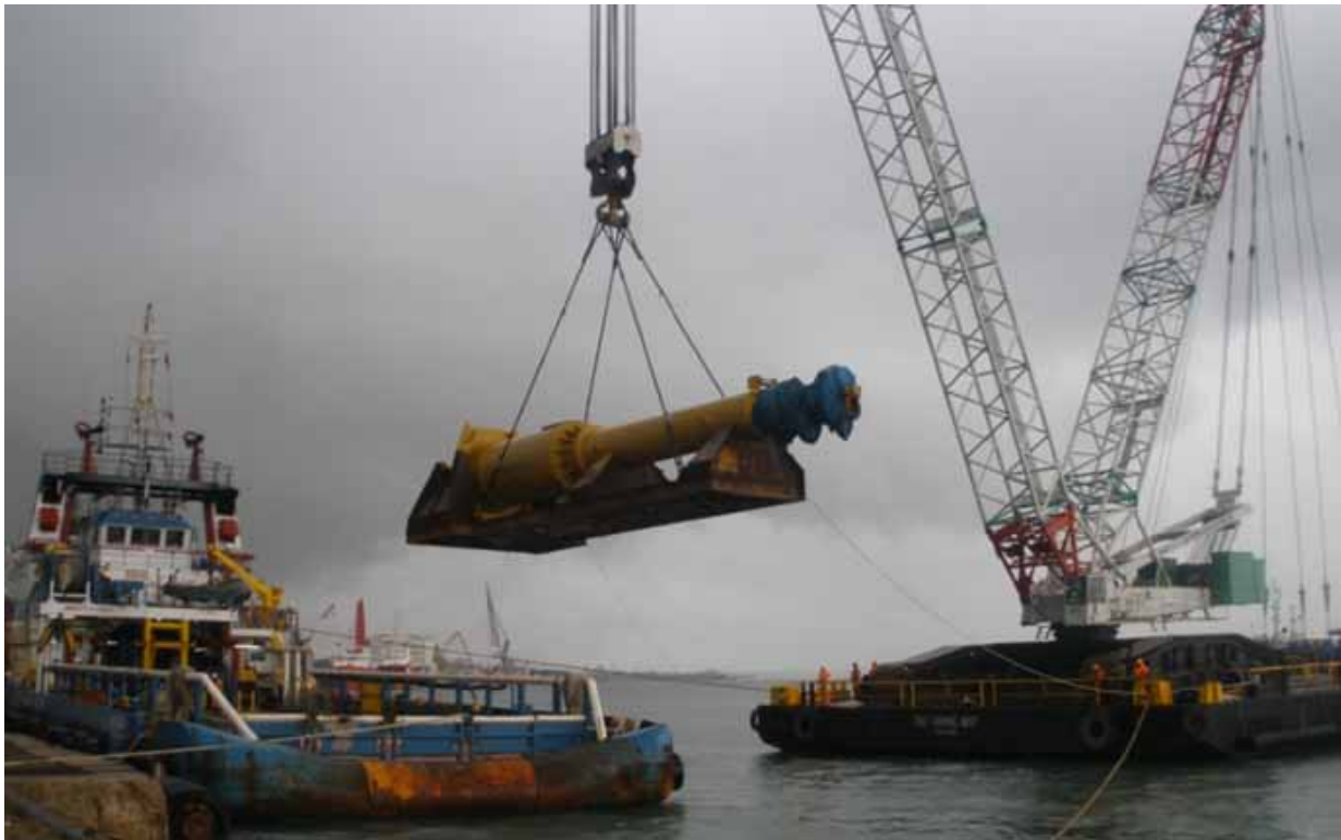
Tat Hong's 817 with Demag CC4000 seen loading piling hammer in Nippon Steel Batam yard Photo : Leen Janse ©
