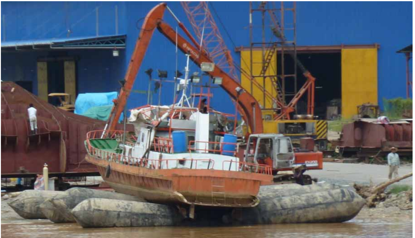
A local vessel is pulled ashore using rubber inflatable bags at a shipyard in Sibul (Malaysia – Borneo)
