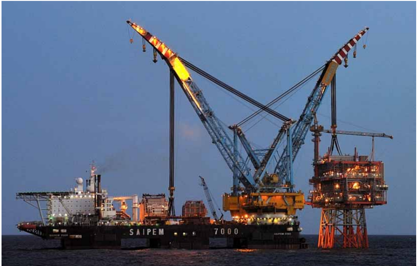
The SAIPEM 7000 seen installing the the Valhall module Photo : Capt. Jan Berghuis (c)
