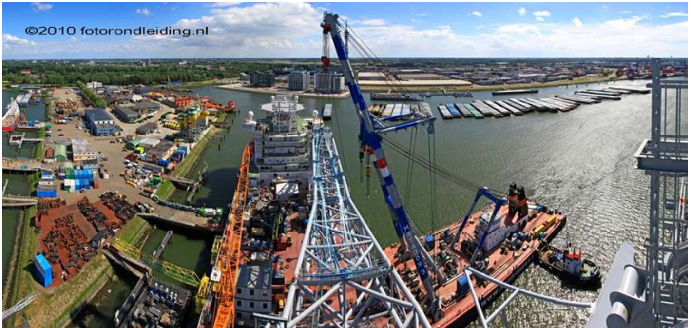
Another photo of the MATADOR 3 seen installing the crane boom onboard the OLEG STRASHNOV
