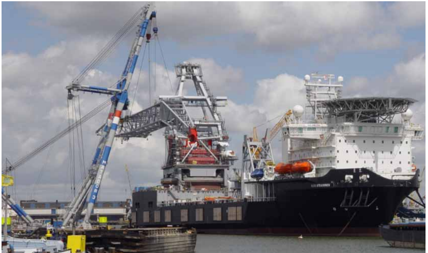
In Rotterdam the sheerlegs MATADOR 3 installed the crane boom onboard the OLEG STRASHNOV Photo : Frans de Lijster ©
