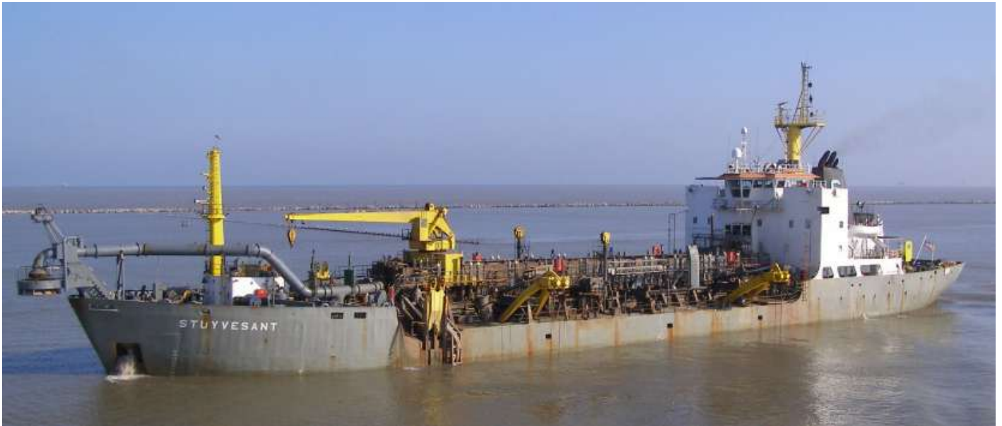
The TSHD STUYVESANT is currently dredging sand in the River and then placing it in a Rehandling Area for the Barrier Island berm project off the Louisiana coast.
