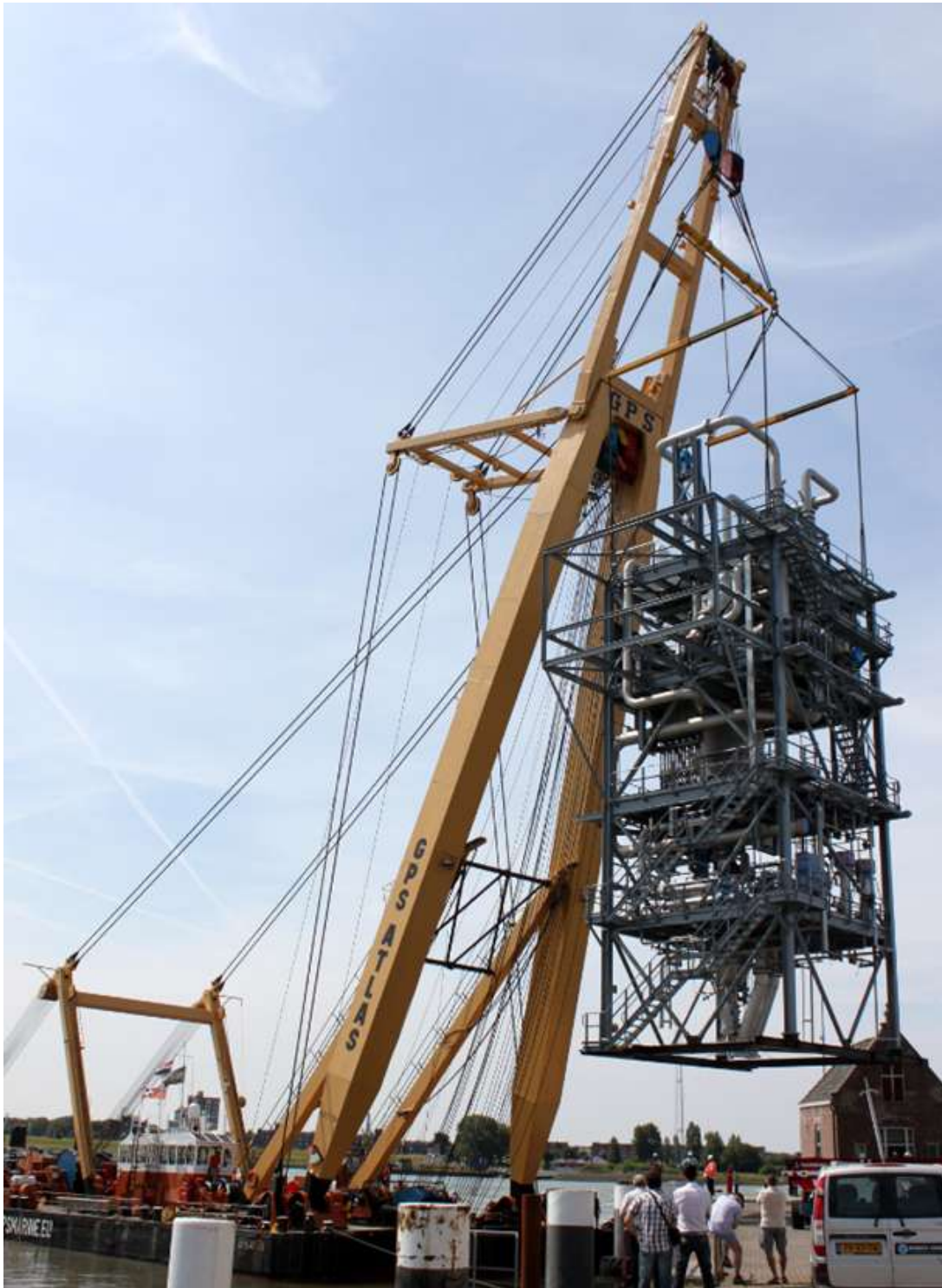
The shearlegs GPS ATLAS collected in Maassluis a filter tower which was built by DAHLMAN in Maassluis and transported the filter to Rotterdam where it was loaded onboard a vessel
