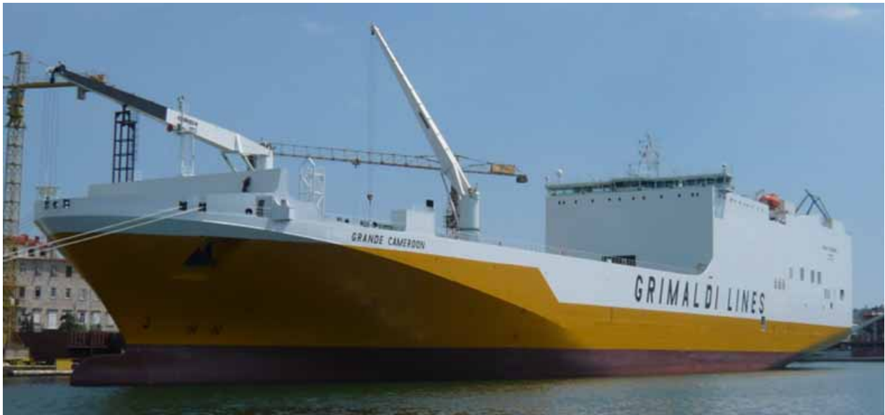
The 26.650 DWT Multipurpose Ro/Ro - Car Container Carrier GRANDE CAMEROON seen ready for departure from the builder, the ULJANIK Shipyard in Pula (Croatia) - Photo : Andre de Vroet (c)
