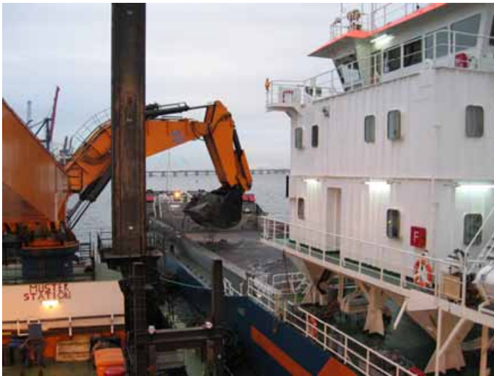
Above seen Backacter Goliath (with 40m 3 bucket) and Jan Blanken during dredging operations in Rio de Janeiro Photo's : Jaap van den Heuvel ©
