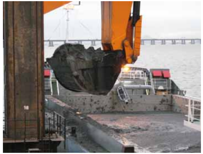
Above seen Backacter Goliath (with 40m 3 bucket) and Jan Blanken during dredging operations in Rio de Janeiro Photo's : Jaap van den Heuvel ©
