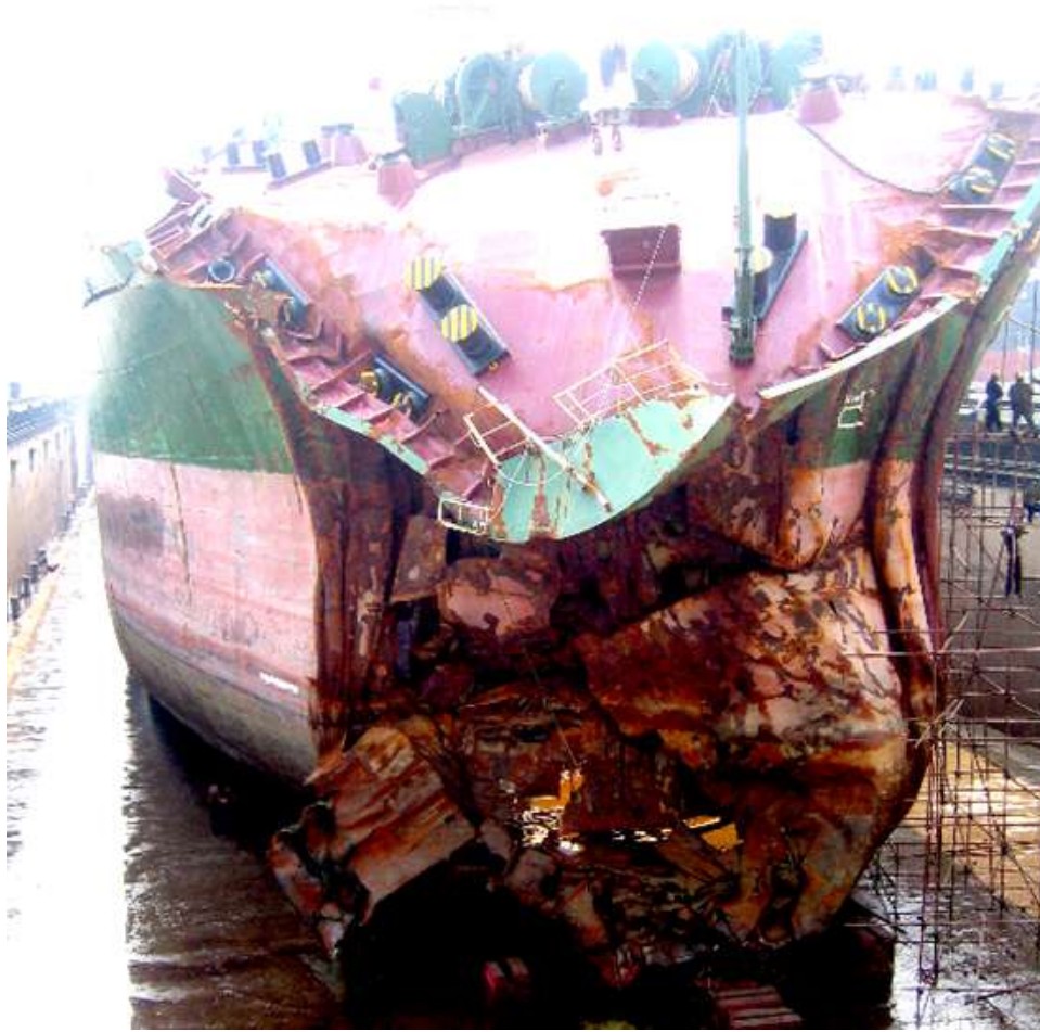
Above seen the SEA SUCCESS in drydock at Xixiakou after a collision with the 178.000DWT Bulker ' Bright Century ' which sunk after the collision.
