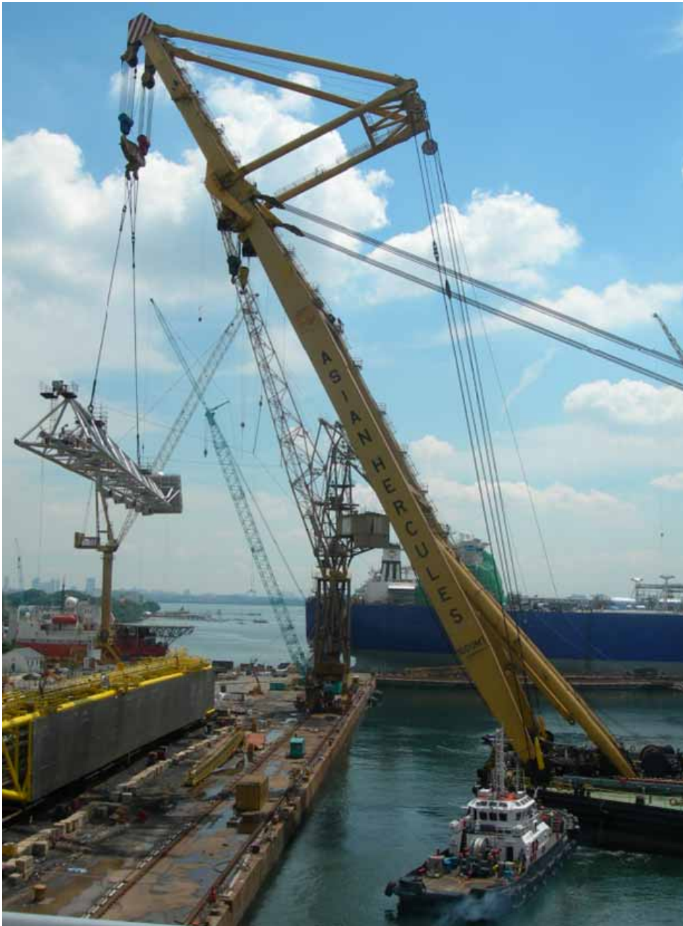
Above seen the 1600 MT sheerlegs Asian Hercules lifting the flare boom tip from the quayside on board the Fjord in Singapore Sembawang - Photo: Jack Geluk ©
