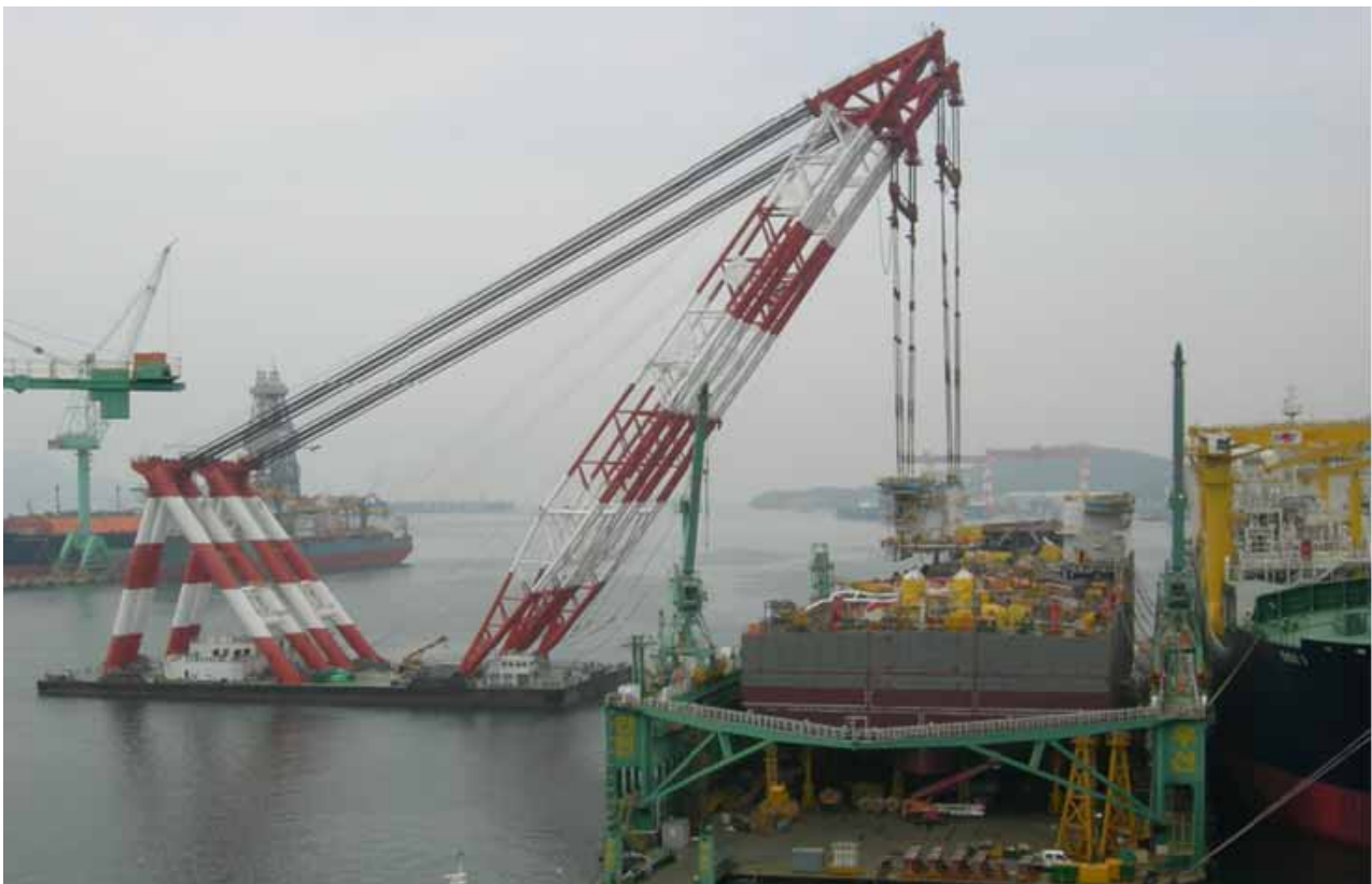
Above seen the Erection subsea module at G1 Floating dock onto Pacific Drilling ultra deepwater drill ship " Pacific Scirocco " at Samsung Heavy Industry, Geoje island, South Korea
