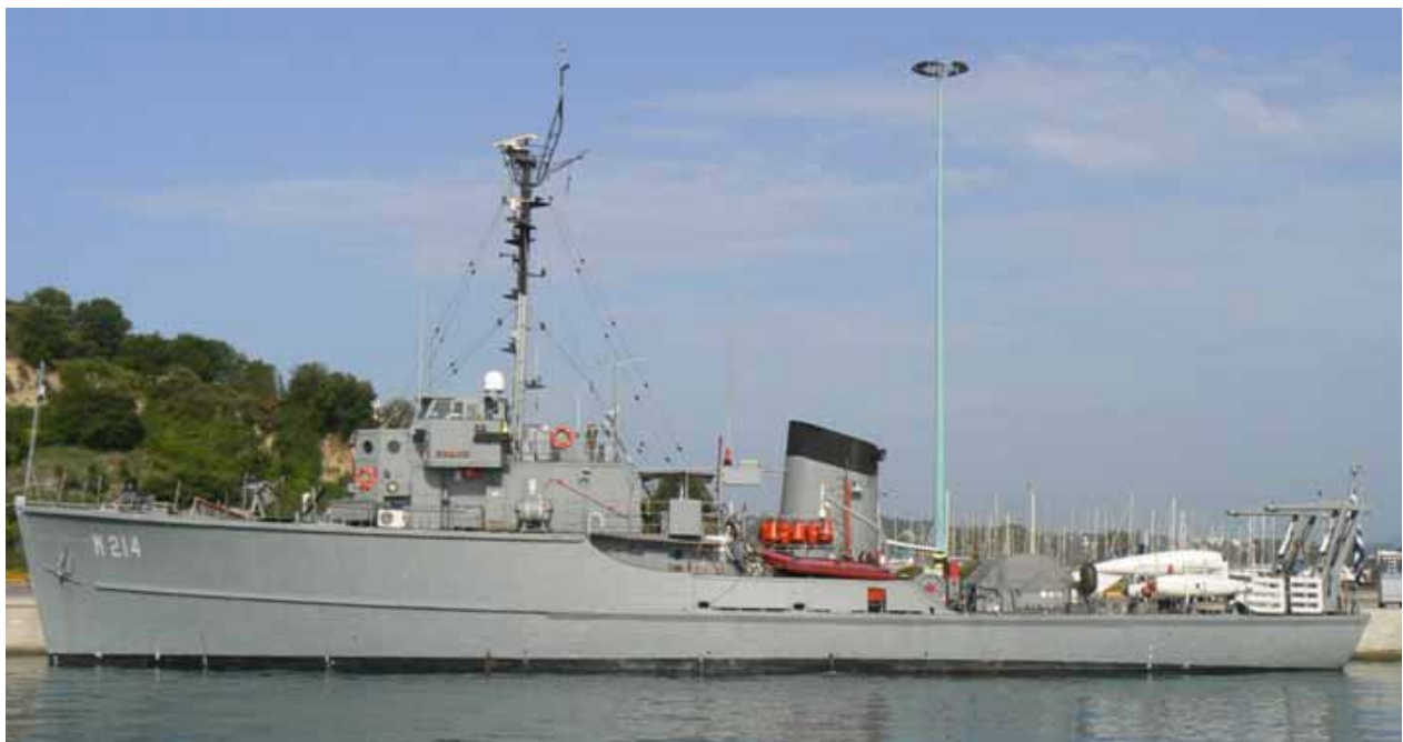
Above seen the 300 ton MSC 214 AVRA (ex MSC 318) one of the 8 U.S. MSC 294–class coastal minesweepers [MSC] built at Peterson Bldrs, Sturgeon Bay, Wis. for Greece under the Military Aid Program; transferred on completion.
