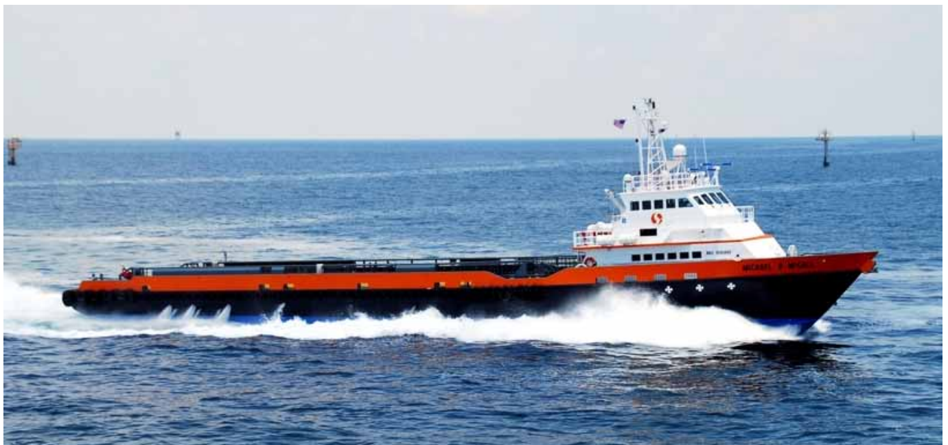
Above seen Seacor's new 57.91M. Fast Crew Supply vessel MICHAEL B McCALL on sea trials in the Gulf of Mexico recently. She is powered by 5 MTU 12V 4000 M60 engines, and has a 370 M sq. Cargo deck.
