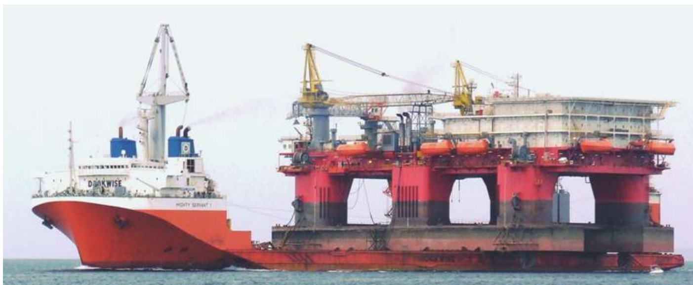
File photo taken December 26 th 2005, of the SAFE CONCORDIA seen as deckcargo onboard the MIGHTY SERVANT 1 out of Port Phillip Bay to Singapore for repairs. Photo : Andrew Mackinnon ©
