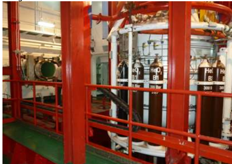
Right : The dive bell with left seen the lock with the chamber(s)
