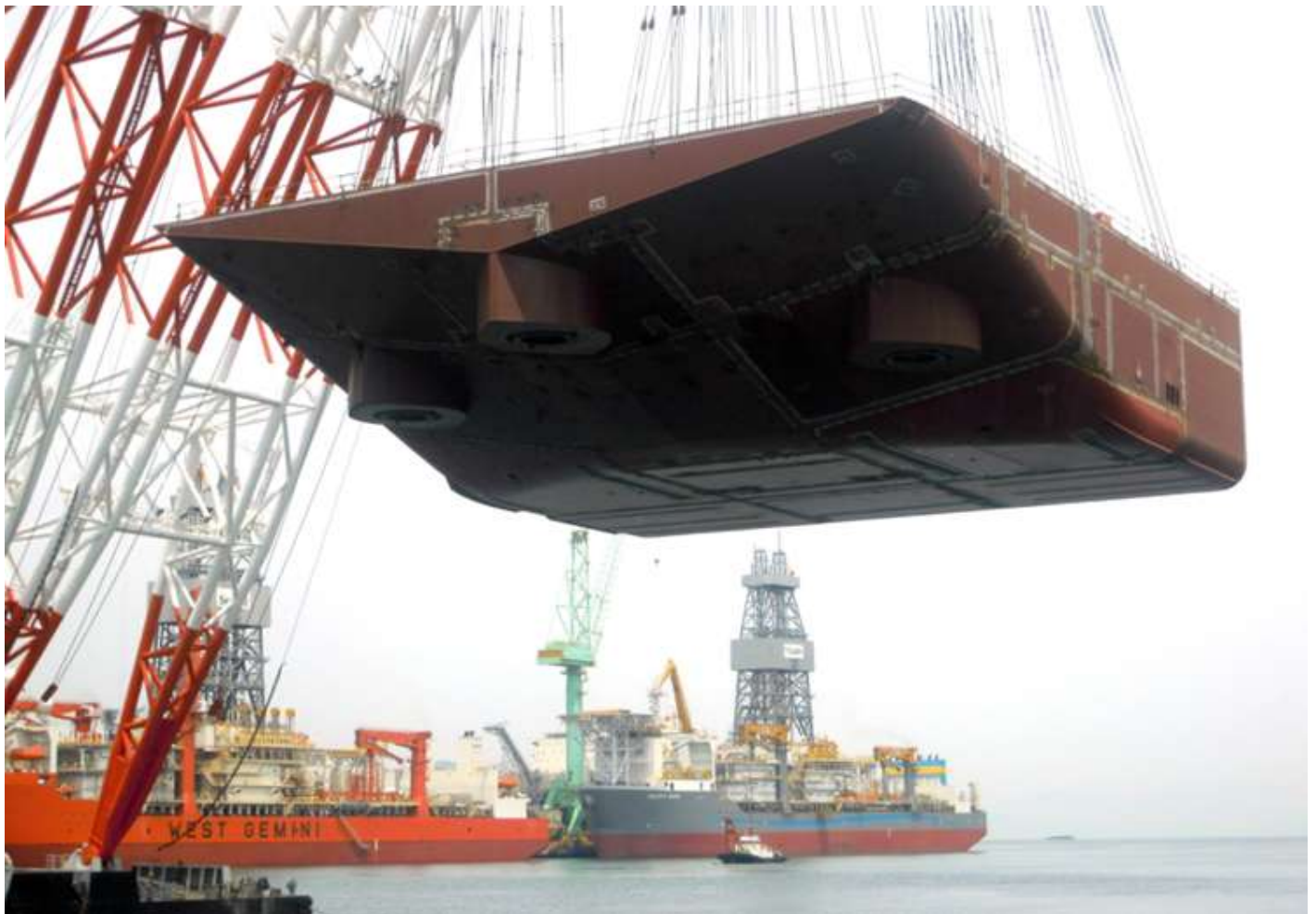
Stern lower half Mega block for ultra Deepwater 12,000 ft Drill ship " Pacific Scirocco " being lifted into Floating dock with " Pacific Bora " and Seadrills " West Gemini " in background at Samsung heavy industry Geoje Island South Korea.
