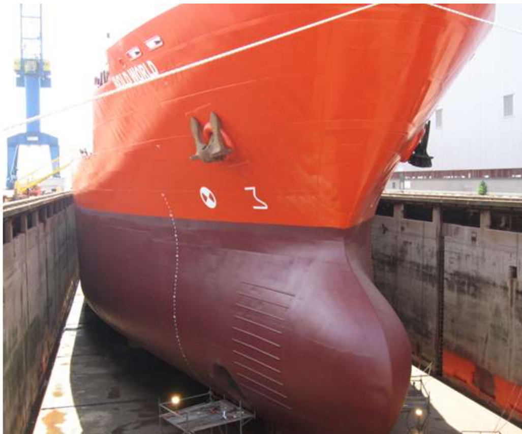
Seen at Scheldepoort in dry-dock at Vlissingen mt " BOLD WORLD " of Messrs Bryggen Shipping & Trading after completion of underwater painting and survey and just before undocking last Sunday
