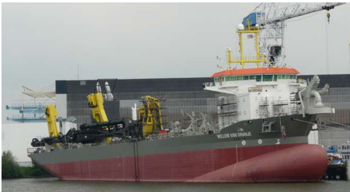
The newbuilding TSHD WILLEM VAN ORANJE seen fitting out at IHC-Merwede
