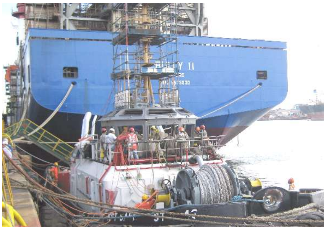
In Singapore the KST SAFE received a new wheelhouse as can be seen above
