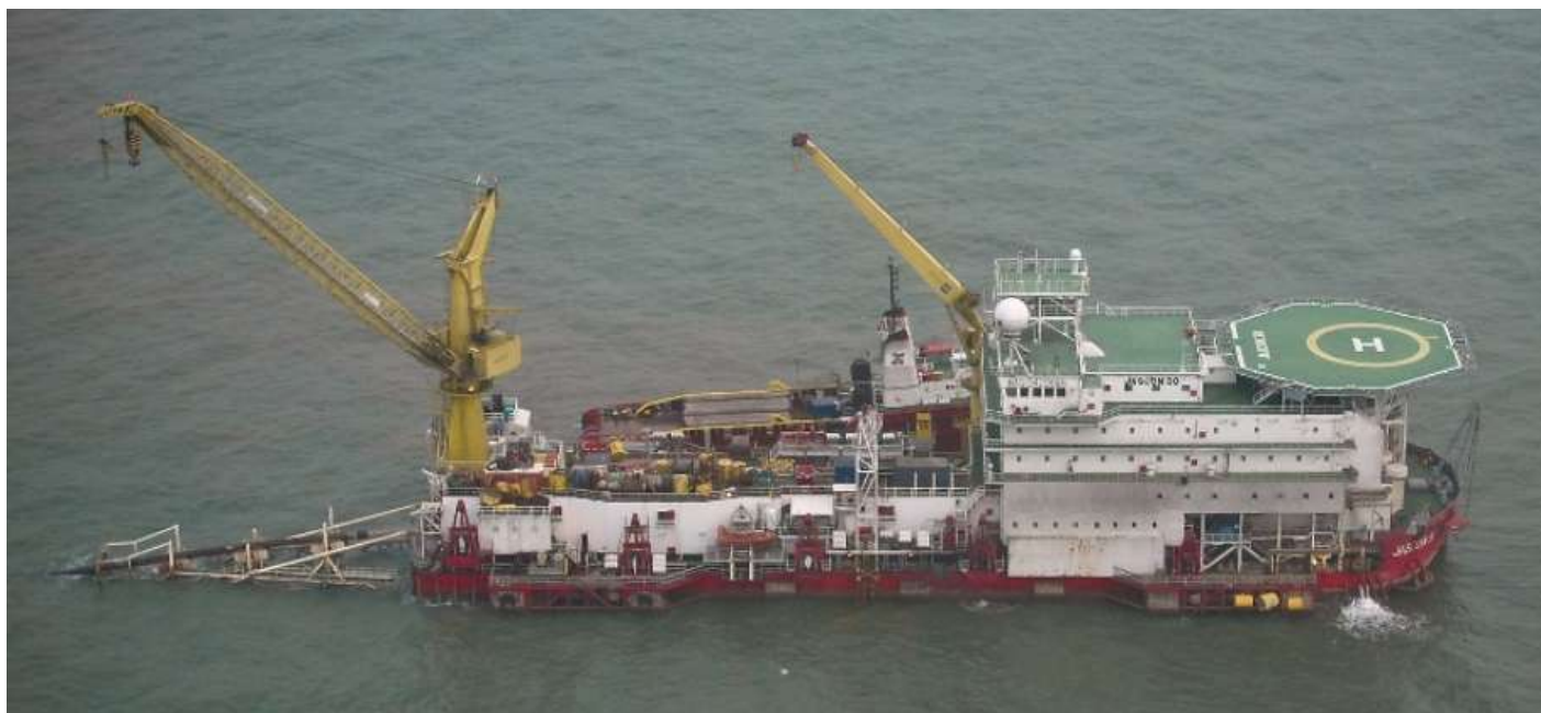
Above and below seen Seatruck's JASCON 30 laying an 24" pipeline for Chevron off the Nigerian coast near Escravos Photo's : Guido de Graaf ©
