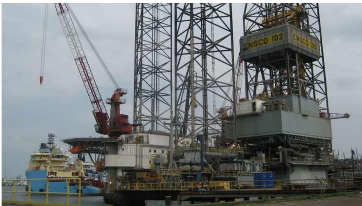
The ENSCO 102 ready for departure from the Keppel Verolme Yard after a cantilever extension job.
