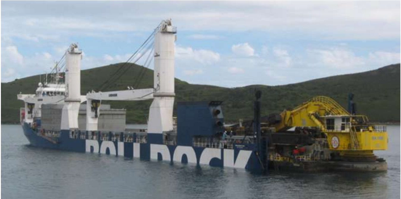
Above seen the submerged Rolldock Sun loading the backhoe dredger Miman Sinan of Jan de Nul in Noumea, New Caledonia with destination Port Hedland in North West Australia.
