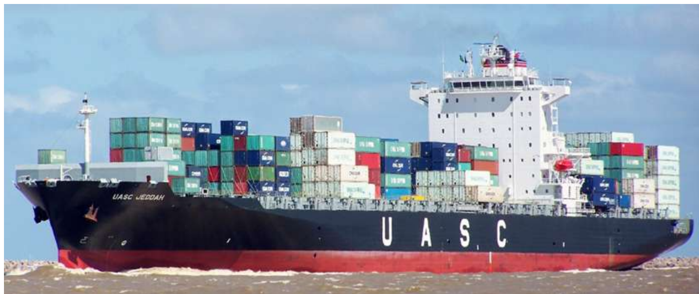
Above seen the 2009 built at Hyundai Samho Heavy Industries Co., Ltd. Ulsan/Korea UASC JEDDAH in Rio Grande, the 262 mtr long and 51.687 DWT vessel is having a capacity of 4255 TEU's and is owned by Reederei Claus-Peter Offen GmbH & Co. KG, Hamburg/Germany and managed by United Arab Shipping Company, (UASC), Dubai/United Arab Emirates
