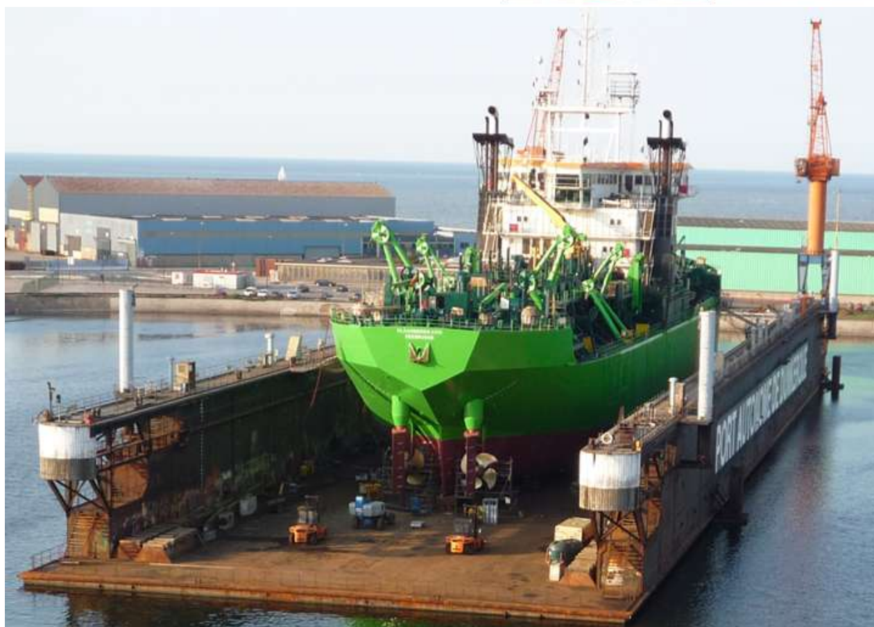
The 1970 built 124 mtr long TSHD VLAANDEREN XVIII seen in drydock at Dunkirk / Dunkerque, the IHC SMIT built dredger with a hopper capacity of 11.300 m3 is owned by Baggerwerken Decloedt & Zoon N.V. from Oostende (Belgium)
