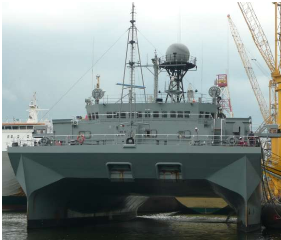
The 1993 built US Naval VICTORIOUS class SWATH ocean surveillance ship EFFECTIVE (T-AGOS 21) seen moored in Singapore – Photo : Piet Sinke ©
