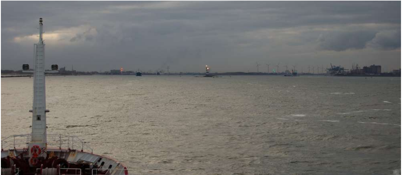
View from the Dutch chemical tanker TOLI (Chemical Tankers Europe Management) whilst approaching the Maasmond, with clearly seen all three leading light lines, the red one on the left for the traffic towards Rotterdam city and the green line for the traffic into Europoort
