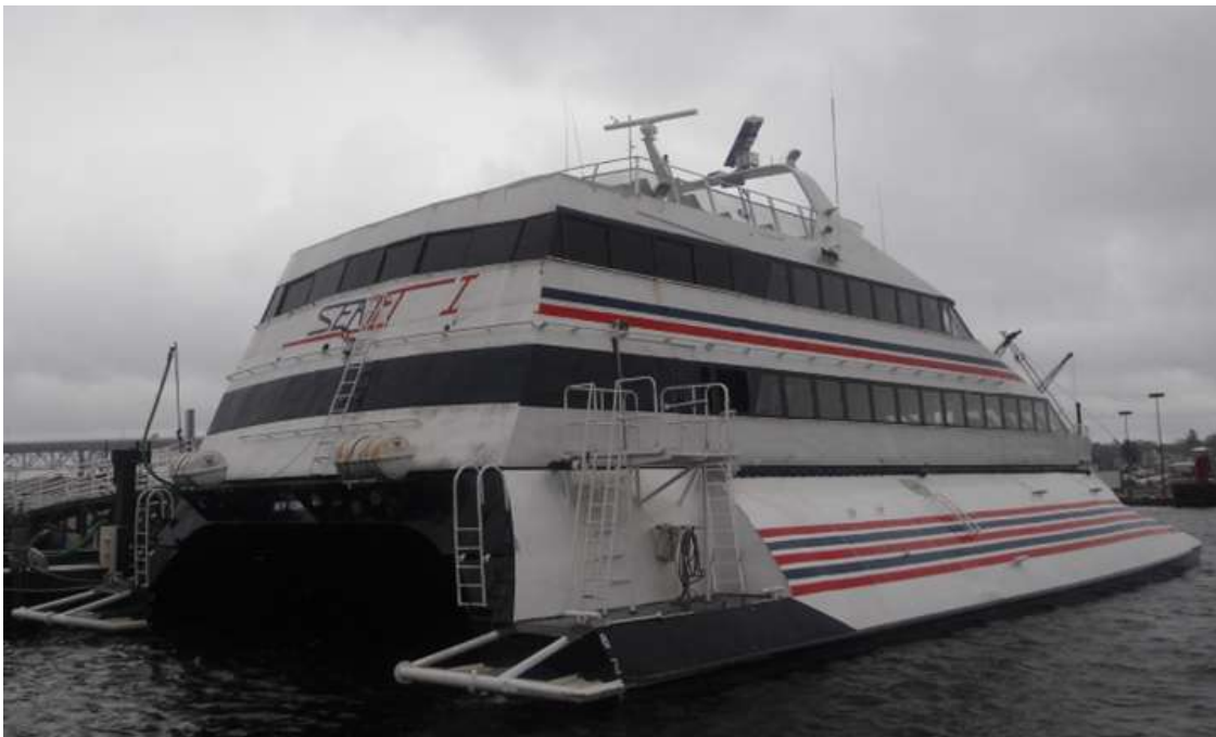
The Cross Sound ferry SEAJET I is having a service speed of 30 knots and 400 passengers capacity
