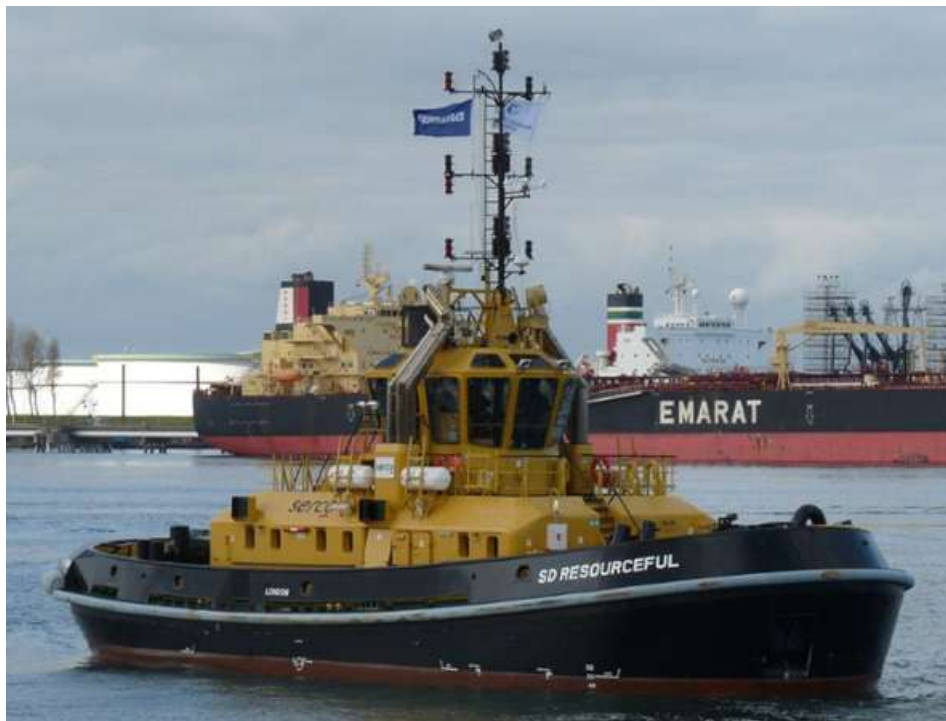
The DAMEN built SD RESOURCEFUL seen conducting bollard pull test in Rotterdam-Caland canal Photo : Frits Janse ©
