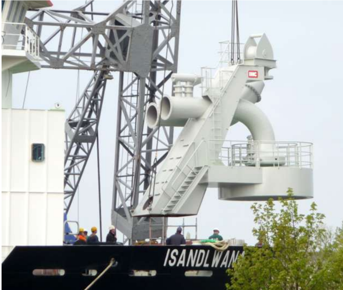
The sheerlegs GPS ATLAS seen installing the bow coupling onboard the newbuild TSHD ISANDLWANA Photo : Jan Oosterboer ©
