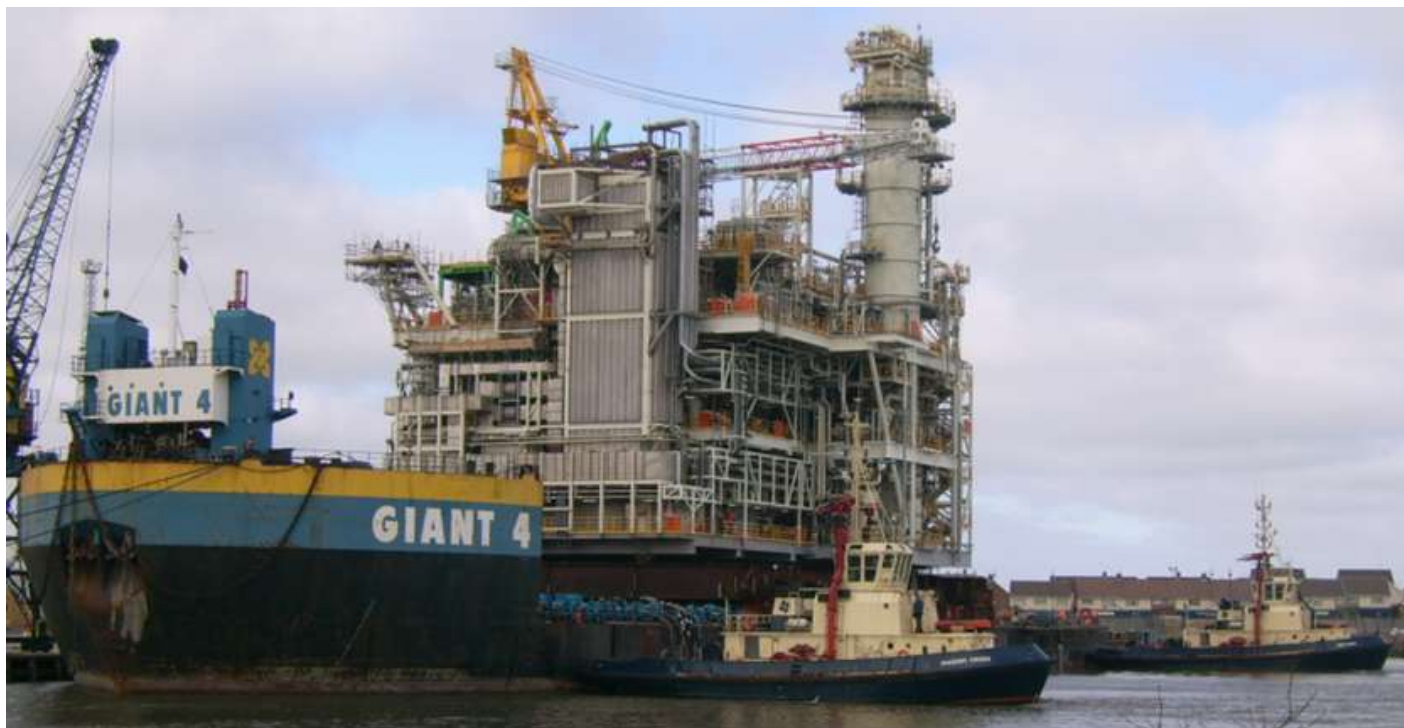
Above seen the GIANT 4 just shifted in the Victoriadock at Hartlepool loaded with the topsite of the Buzzard with a total weight of 7000ton which will be discharged by the SAIPEM 7000 op at the location
