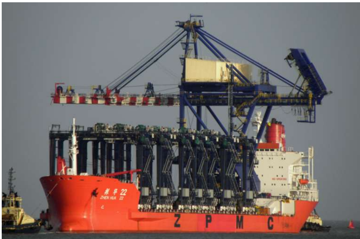
The arrival of the Zhen Hua 22 at Felixstowe April 15 th evening assisted by Svitzer Melton and Svitzer Shotley she has RTG's for Felixstowe. The ship to shore crane is for delivery to Rouen.
