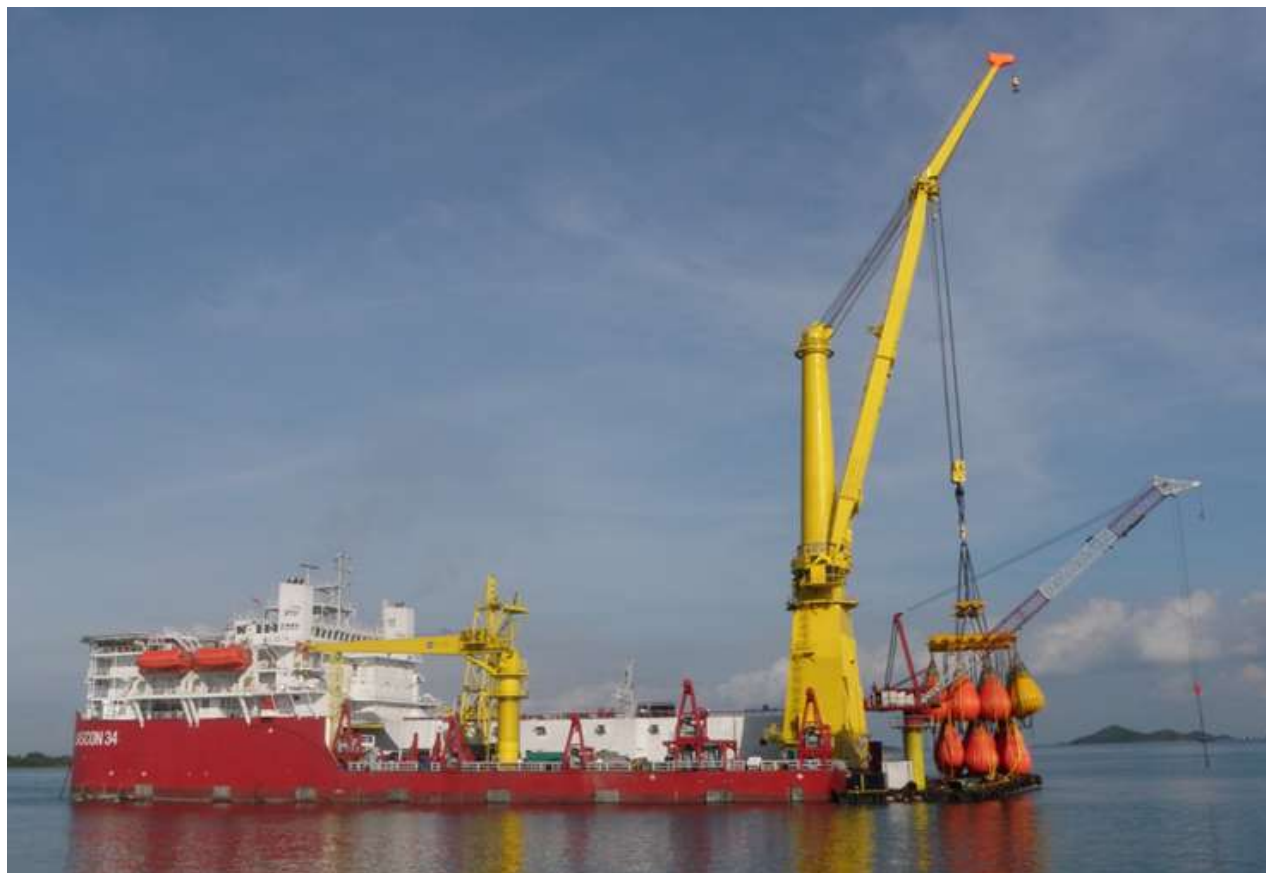
The Jascon 34 preparing for loadtesting an 800 mT Huisman crane in Batam.
