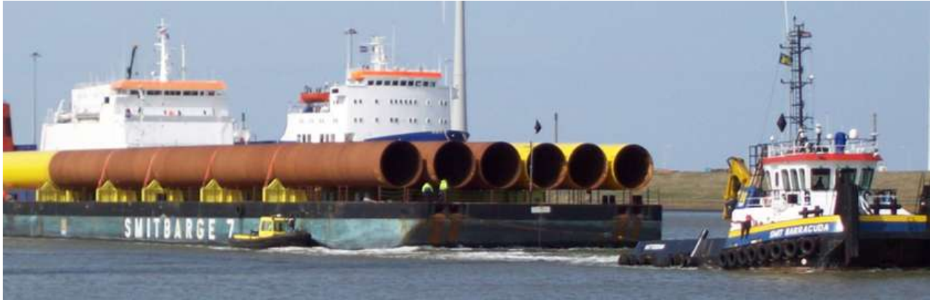
" Smit Barracuda seen towing Smit Barge 7 , departing from Eemshaven, loaded with the first windmill piles for the BARD Offshore 1 project approx. 100 km. offshore in the German Bight"
