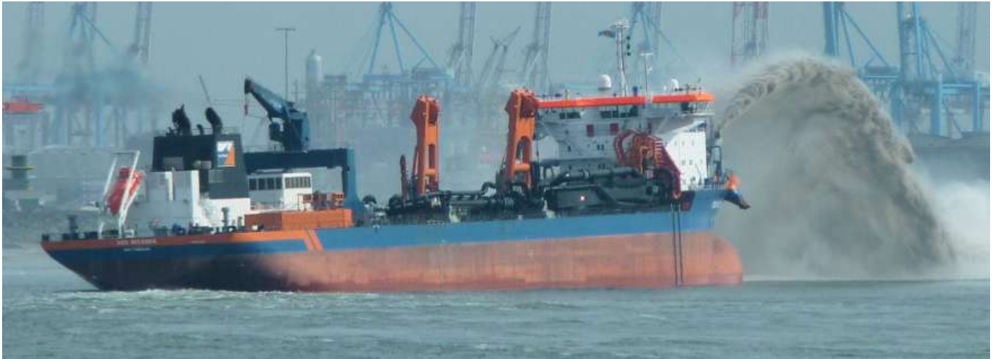
The VOX MAXIMA seen rainbowing at the Maasvlakte 2 project - Photo : Marijn van Hoorn (c)
