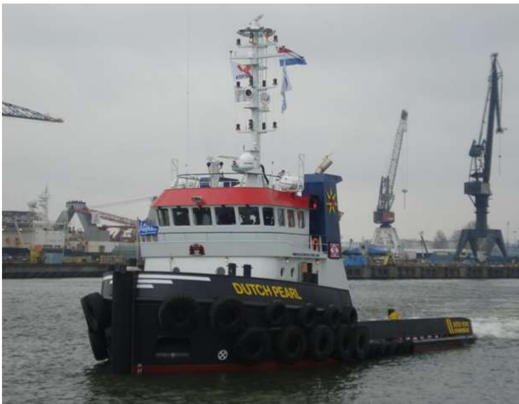
The DUTCH PEARL seen conducting bollard pull tests in Rotterdam-Botlek - Photo : Bas van Hoorn (c)
