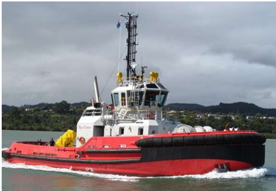
Above seen Rio Tinto's latest new build departing from Shipco in Whangarei, New Zealand bound for Cape Lambert in the Pilbara, Western Australia. Oita is a 32m 65t bollard pull Robert Allan designed ASD tug
