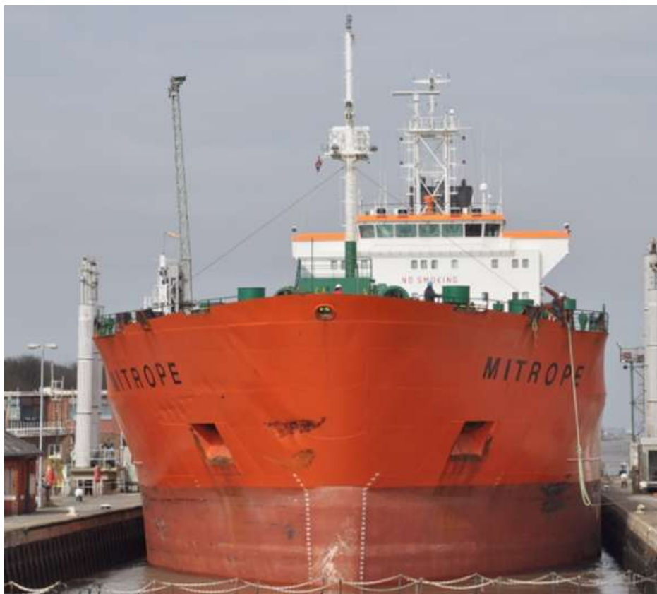
The 1999-built molten sulphur tanker Mitrope entering Eastham Locks on the Manchester Ship Canal. The lock is 24.38m wide, whilst the ship is 23.16m wide.
