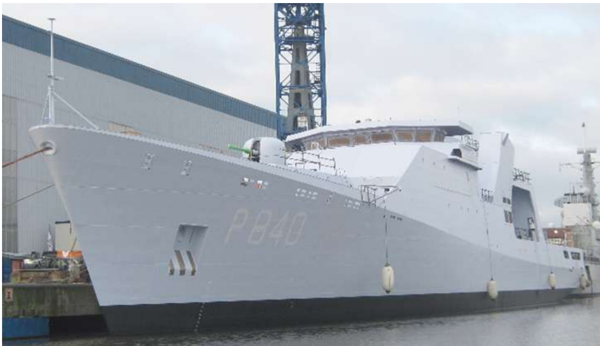
Above seen the P 840 HOLLAND fitting out at the Damen / de Schelde Naval yard in Vlissingen Photo : Damien Benthem ©
